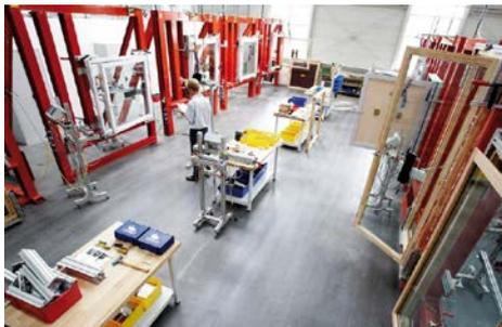
In the certified test centre Roto ITC – International Technology Centre – in Leinfelden, window and hardware tests for individual project solutions are properly carried out to national and international standards. In this way, individual warranty extension prerequisites are also created.
