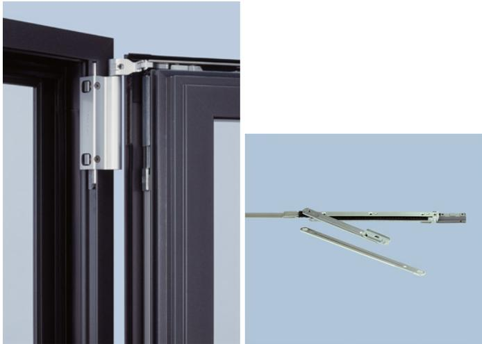
Roto developed tilt and turn special solutions for the Hamburg 'Dancing Towers' window sashes: A modified locking scissor stay that can hold a weight of some 65 kg per sash in opened turn mode, even where the facade inclines outwards or inwards, was combined with Roto AL series turn-only hinges and locking components.
