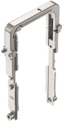
Thanks to a special corner drive specifically developed by Roto, the ventilation flaps which are integrated in the facade in addition to the Turn-Only windows are locked all the way round their circumference. This improves the sealing of the closed ventilation flap and therefore the thermal insulation in the facade.
