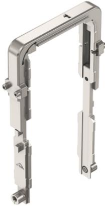
Ventilation flaps are locked around their circumference by a specially developed special corner drive. This improves the sealing of the closed ventilation flap and therefore the thermal insulation in the facade.
