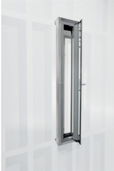
For the most popular opening type, turning, Roto made it possible to limit the travel and opening angle of special hinge sides based on the “Roto AL Designo” in such a way that the ventilation flap virtually has an integrated opening restrictor. In this way, the opening width of a ventilation flap can be individually restricted on request, therefore preventing damage to the fittings or adjacent components, for example.
