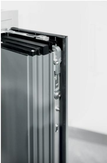
For high-quality ventilation flaps, Roto recommends the use of special corner drives which allow active locking points to be set on the hinge side by means of a connecting rod. This makes it possible to produce tightly sealed flaps, which can be suitable for RC 2, even where space is limited in the rebate of narrow sashes. At the same time, these active locking points counteract sash warpage, which can become a problem with ventilation flaps.
