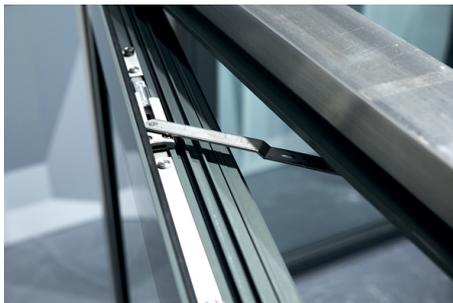
The robust solution for protecting high-quality aluminium Turn-Only windows: using Roto's innovative opening restrictor makes it possible to open a window sash up to a defined opening width and lock it in the end stop position simply using the handle.
