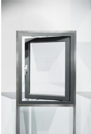
New for aluminium windows: the lockable opening restrictor from Roto. The sash is locked by moving the handle at the end stop from the 90° position back into the 0° locked position. Only authorised staff are able to unlock the handle using a removable key on the cylinder when the sash is closed and disable the turn restrictor by turning the handle to 180°.
