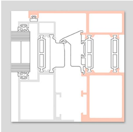
Profiles for a window that is flush with the surface must offer a 17.5 mm rebate clearance for the hardware instead of the usual 11.5 mm in the Euro-groove. This is the only way to fit a user-friendly hardware configuration for sashes with a high weight.
