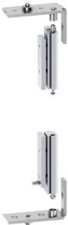
Roto Aluvision configures property-specific heavy-duty hardware for profiles flush with the surface that achieve a load of up to 250 kg sash weight. The image shows the pivot rest and corner hinge at the top and bottom. In the case of high sash weights, they are attached using special self-tapping screws.
