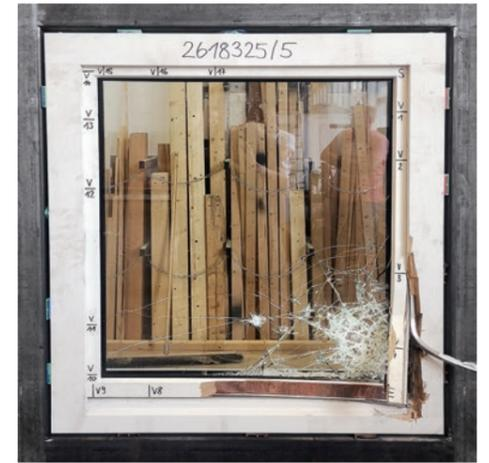
Element from Hans Timm Fensterbau GmbH following the RC 4 test. Bastian Timm is satisfied: "The security components from Roto helped us make an extensive range of timber windows fit for the RC 4 tests. The tests were passed on the first attempt."
