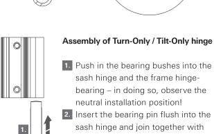
2. Insert the bearing pin flush into the sash hinge and join together with this the sash hinge and the frame hinge-bearing.
