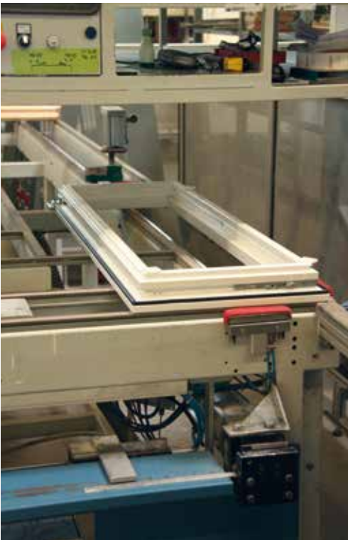
swisswindows has been cooperating with Roto for 25 years. Pictured: automatic installation of the Roto NT hardware.
