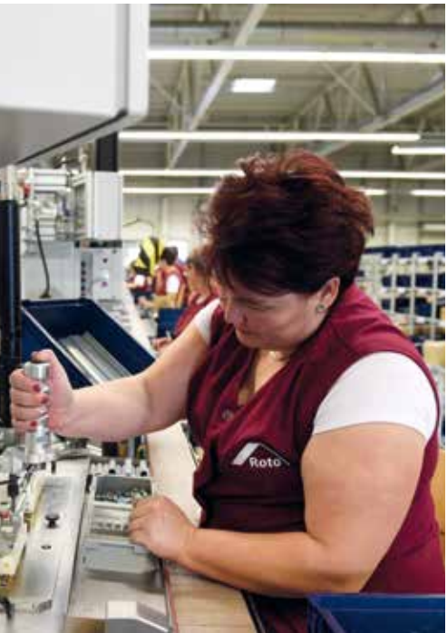
The assembly line works with the latest screwing and pressing technology for a wide range of applications. The forming pressure is set automatically after the product code has been scanned. A press stroke measuring system then checks whether a frame-hinge pin has been pressed as required.
