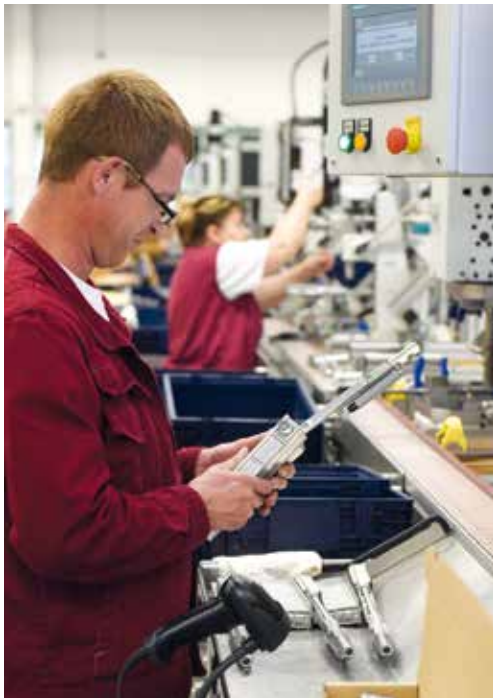
Because not all assembly stations can be timed synchronously, the specialist staff look after two fast stations simultaneously or one slower one. All employees are adept at working anywhere on the entire line. A comprehensive final inspection is carried out before the bogies are packed into a custom fit cardboard box.
