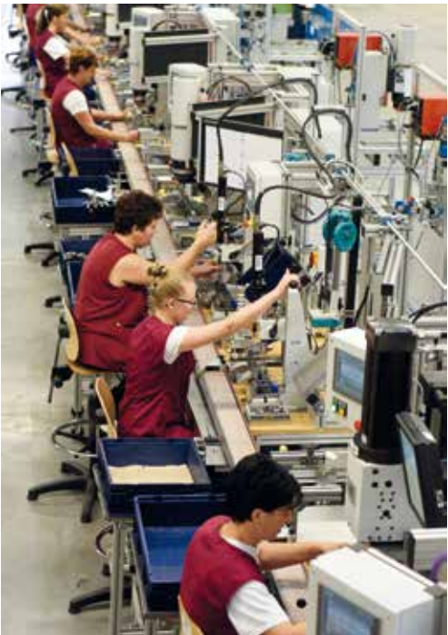
Line 81 in L  v   is where bogies and scissor-sliders are made for the Roto Patio Alversa parallel and tilt & slide system. About 400 standard items have to be mastered in assembly and order picking. About 300 separate order-specific parts are assembled for each consignment.
