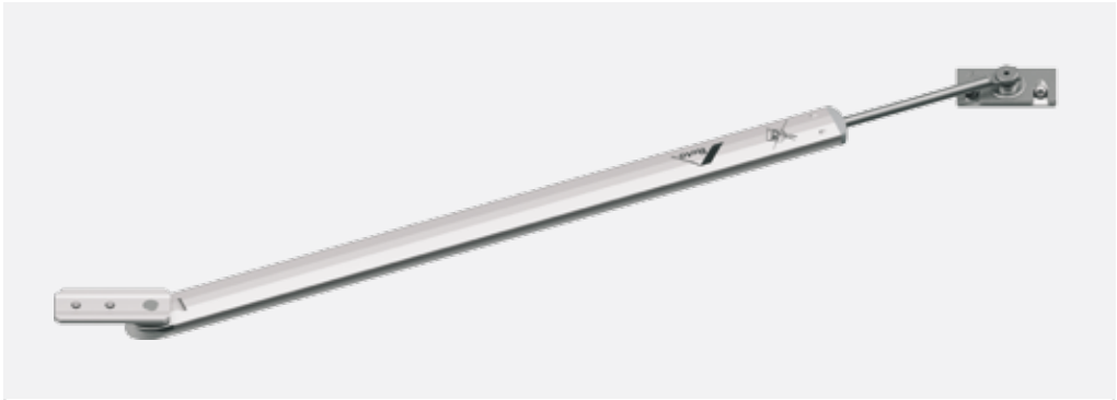
This 2.1 opening restrictor’s braking force is preset and optimally matched to both hardware ranges’ hinge-side components. It has a test certificate in accordance with DIN EN 13126-5 application 5/1 and is classified as a “limiting restrictor”.
