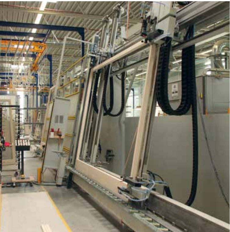
The introduction of the frame press led to a halving of the cycle time, a further sustainable quality improvement and a substantial reduction in staff deployment.
