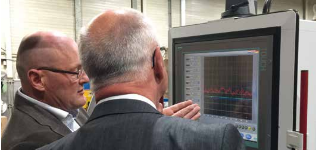
In order to be able to supply seals for every application, Deventer Profielen B.V. extrude both from foamed TPE and TPV, and to a limited extent, also from PVC. Production manager, Jeroen Mols (pictured left) explains to the Chairman of the Roto Frank AG Board of Directors, Dr Eckhard Keill, how quality control is set up during the extrusion. Production quality is controlled where the seal is formed, but also where it is packed.
